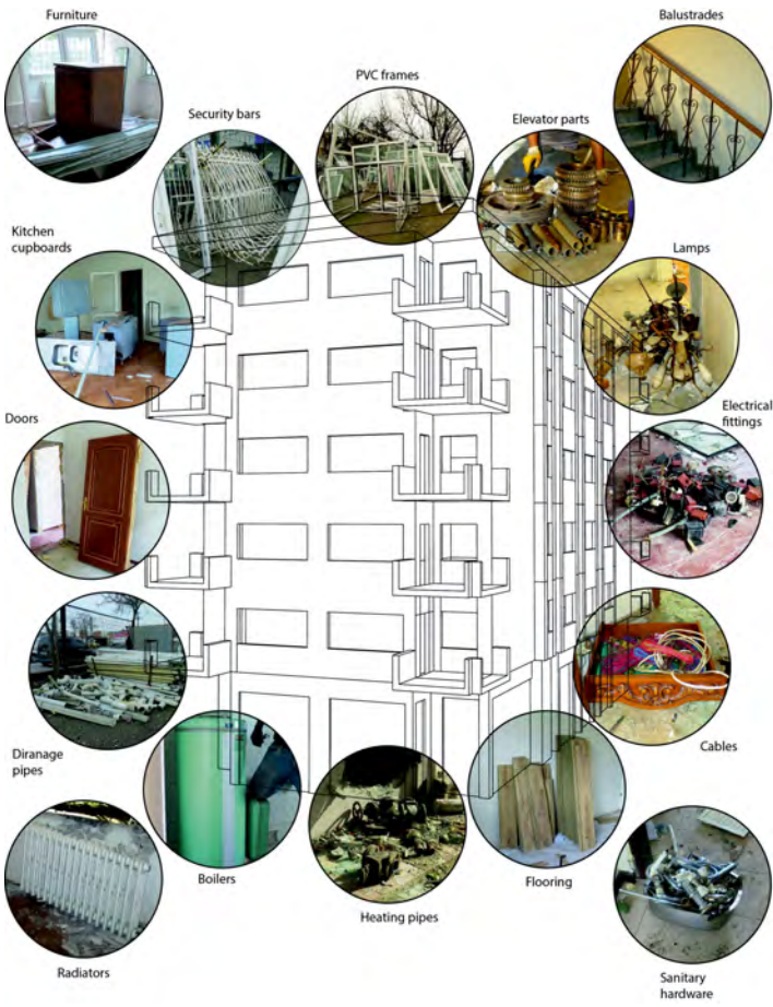
Figure 5.1: Building elements recovered from an apartment
