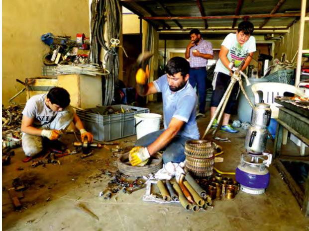
Figure 5.11: Dismantling elevator parts 15
